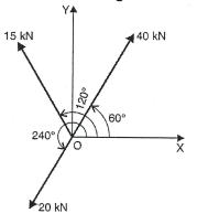
Find the resultant of the force system shown in Fig. acting on a lamina of equilateral triangular shape.
