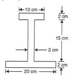
Find the centre of gravity of the I-section shown in Fig.
