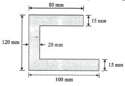
**SECTION – VI** Determine the moment of inertia about the centroidal axis of the following crosssections. Also find the radius of gyration. All dimensions are in mm.
